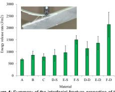
Figure 4: Summary of the interfacial fracture properties of the sandwich structures
