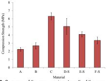
Figure 3: Summary of the compression strength of the core materials
